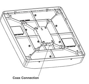
Figure 3 Antenna and Mount Assembled
